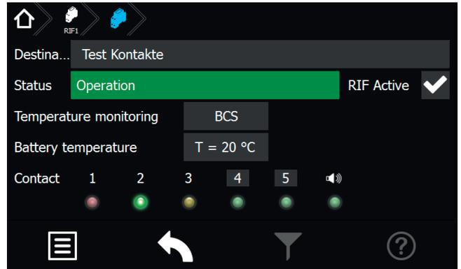
The upper area shows the allocated destination text and the current device status. A combo box offers you the following choices for a temperature-controlled charging:
