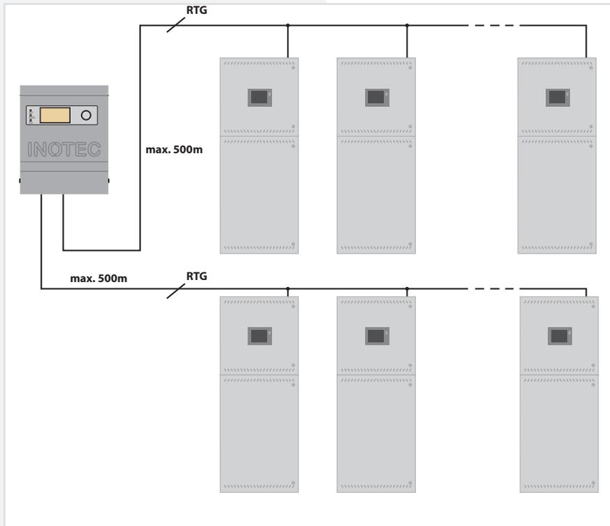
Max. wire length with 0.5mm<sup>2</sup> (minimum cross-section) 500m.
