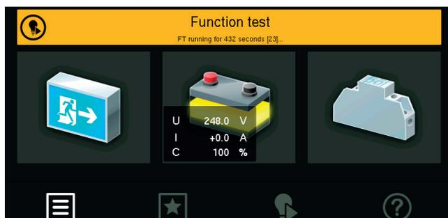
In FT mode, the device switches to battery operation and checks the operability of the connected and activated luminaires. The result of the FT is stored in the logbook. The current system status appears in the “status display” on the main screen.
