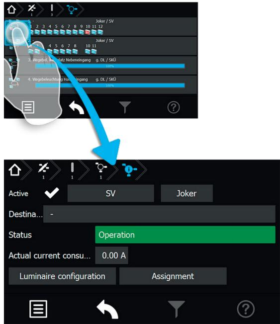
The sub-menu of each final circuit contains status information. The type of monitoring and operation mode can be selected in the two combo boxes on top. Furthermore, the destination text, the status and the actual current consumption of the final circuit can be found here.
