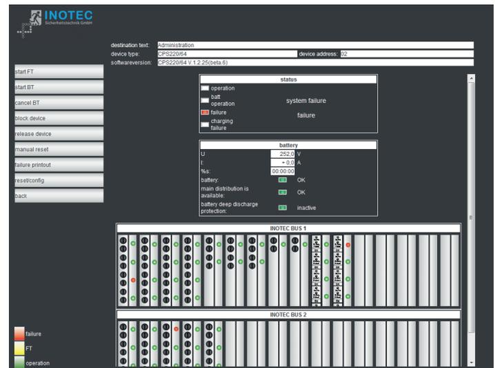
The status information of the luminaires can be displayed via the INOWeb interface using a web browser. To that end, the CPS FUSION is integrated into a local network.
