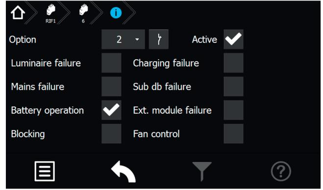
You can assign the switching mode (normally closed or normally opened) in this dialogue window. You can also assign the message type here.
