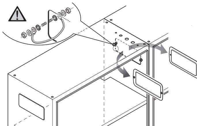
For fitting batteries in two or more battery cabinets, the side flange plates must be removed to enable wiring as shown in the diagram.
