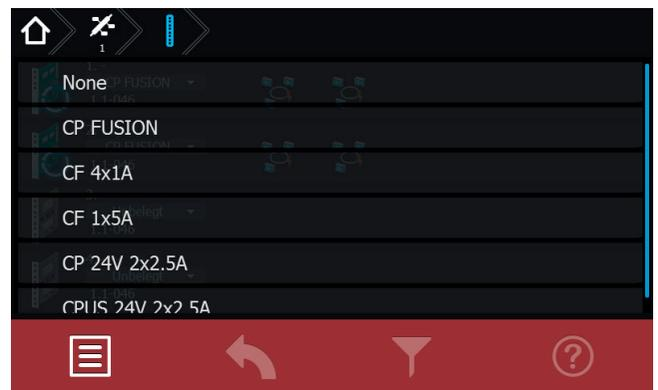
To program a luminaire select the related circuit and go to the luminaire level. Luminaires can be selected / unselected via dropdown menu.
