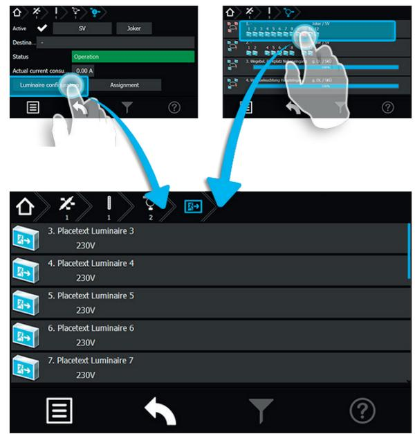
Another way to access the “luminaires” sub-menu is to select the “activated luminaires” button in the “final circuits” menu.
