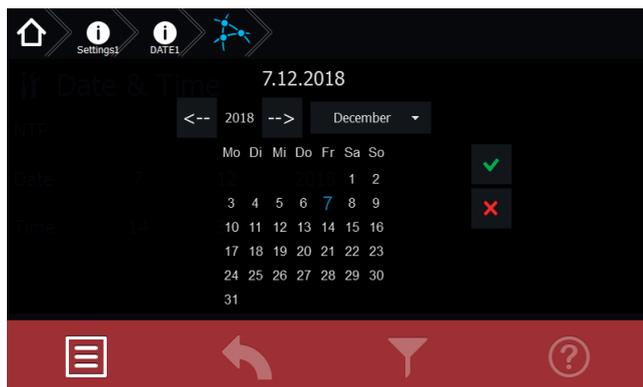
The upper line of the dialogue window displays the chosen date. The middle of the screen shows a calendar. The month and year can be set up by the arrow button.
