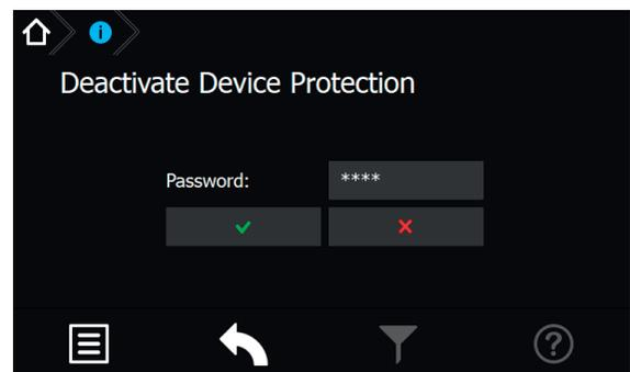
After entering the correct password, access to the controller is enabled.
