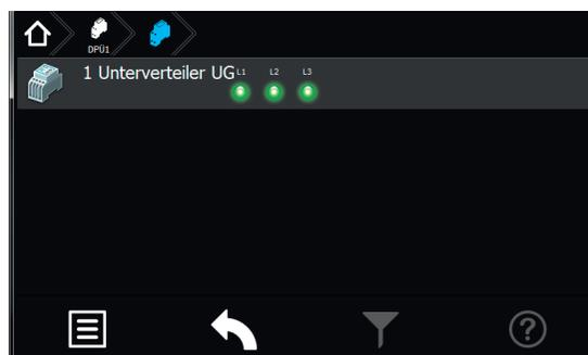
The DPÜ/B modules are directly installed into the sub-distribution boards to monitor the supply voltage of the general lighting. The modules are communicating by BUS line IB2 or IB3. Up to 31 pieces can be connected to the BUS. If a phase fails, this will be indicated at the controller.
