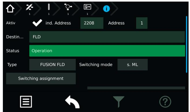
In case of 24V luminaires, the individual address and the freely programmable address can be found in the two upper fields. Operating status, luminaire type and entered destination text are indicated in the corresponding data fields. The operation mode and the measured current are given in the lower information displays.
