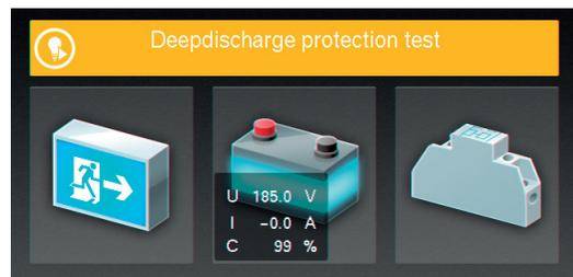
Once the test procedure has been completed, the lowest voltage value remains visible for a short period. The battery icon changes back to green if the interruption was OK.
