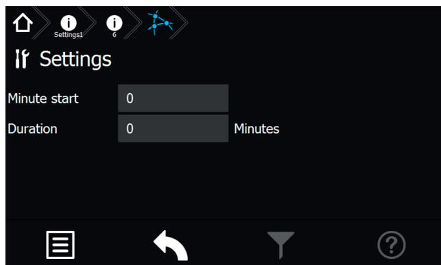
The start time (in minutes) is set by the "Minute start" button. The duration is set by using the "Duration" button.
