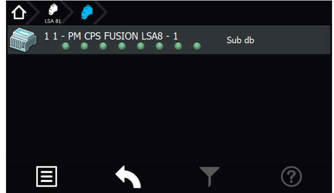
The LSA8 and LSA 3.1 modules can be used to switch the general- and emergency luminaires simultaneously. Up to three switch inputs can be assigned to every final circuit.
