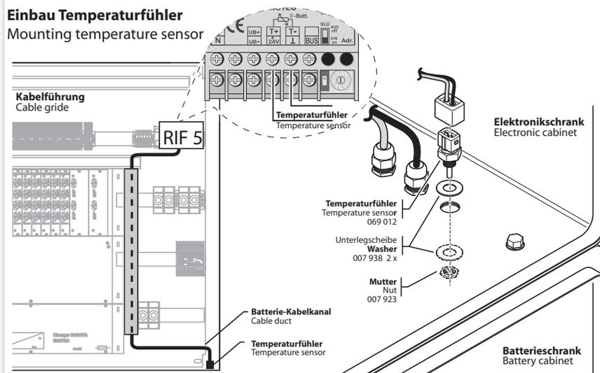
For the battery cables and the optional temperature sensor, the three screw connections (for battery sets connected in parallel, five screw connections) are to be mounted between the electronics cabinet and the battery cabinet. If no temperature sensor is used, the third screw connection must be sealed off with a blank plug (supplied).
