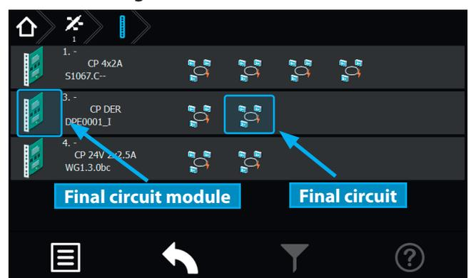
You are now at the level of the change-over devices. The SKUs are arranged vertically on the left side of the menu. The module slot number and the type of SKU can be found on the right, next to the change-over device icon. The circuits of the SKUs are arranged horizontally on the right of the menu.
