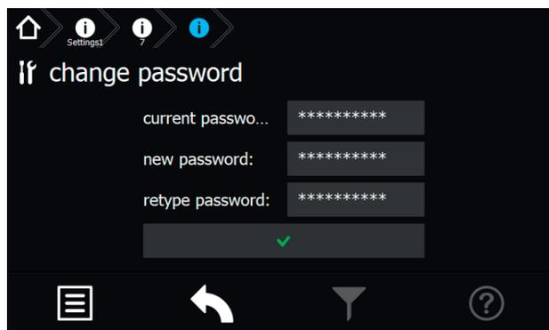
To assign a new password, the current password must be entered first, followed by the new password and confirmation.
