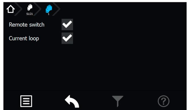
This sub-menu displays detailed information about the SLÜ module (separate module or integrated into the RIF5 module). Two check boxes indicate whether the respective monitoring mode is activated or deactivated.
