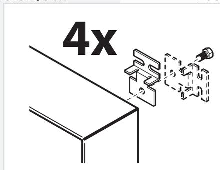
The electronics and battery cabinets are placed on top of each other at the assembly site and connected with the screws supplied. To guarantee the required clearance to the wall, the cabinet is fastened to the wall with the wall-mounting straps provided.
