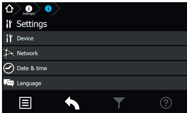
The “Settings” menu gives you the possibility to change the programming of the device. It’s possible to change the network settings, automatic test settings, fan-control settings and date and time settings in this menu. In addition, in the “Learn Mode” area, the desired monitoring mode can be set and an individual password can be assigned in the “Password” area.
