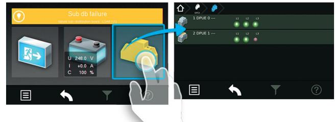
Submenu will show information about all connected DPÜ/B modules including their locations when you activate the button „Components“. All phases which were detected as a power failure will be highlighted by red LEDs in the submenu „DPÜ/B“.
