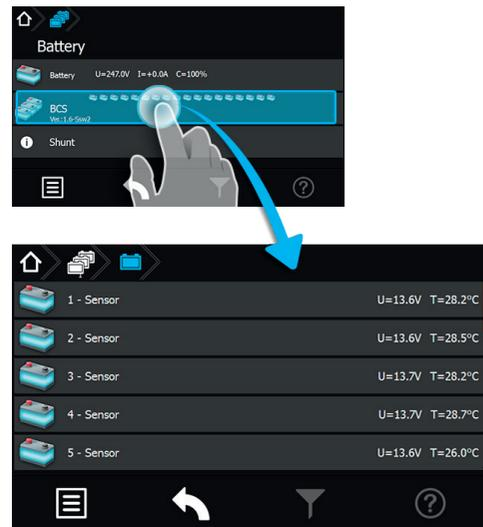
Each sensor is displayed in a separate column, showing the current values of the monitored battery block. The individual voltages and the temperature of the battery blocks are displayed here. It's not possible to open the columns of the individual sensors.
