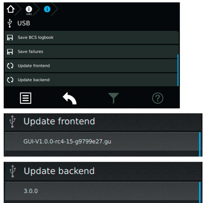
Selecting this file will copy the new software to the controller. An automatic reboot will load the new software.
