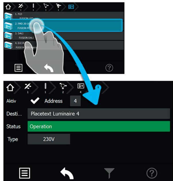
This menu allows you to activate or deactivate individual luminaires, by using the  „activated“ or  „deactivated“ buttons.
