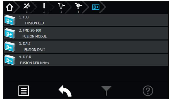
A destination text is shown on the respective luminaire button, if entered. If more than one luminaire is activated on a final circuit, they are displayed one below the other.
