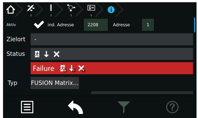
For dynamic luminaires, the actual LED matrix status is displayed in the status field. This depends on the active switching inputs and programming.
