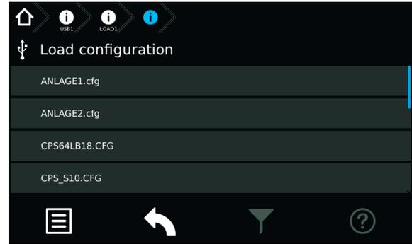
A list with all available configuration files will be shown on the screen. You can load the needed file by clicking on the corresponding button.
