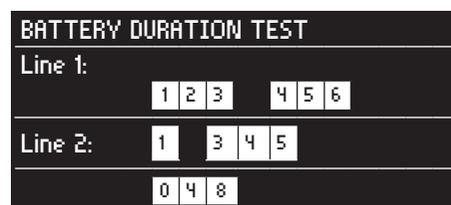
The following screen shows all panels that are in duration test mode. After 2 minutes the duration test can be canceled.
