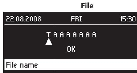
The file name consists of 8 letters or digits. Turn the control knob to select the desired letter or digit. Press the control knob to confirm the entry and move the cursor to the next position. After entry, press the knob again to confirm the name.
