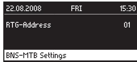
Turn the control knob to change the RTG address for the BNS-MTB and then press the knob to save the address.
