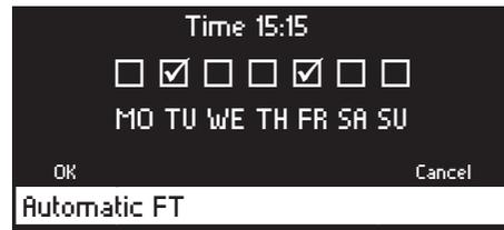
Turn the control knob to select the time or a particular weekday. To make a change, press and then turn the control knob. Pressing the control knob again takes you back to the selection screen. The selected weekdays are marked with a tick. An automatic function test will be performed at the set time on these days every week. Press „OK“ to confirm the changes or „Cancel“ to exit the menu without making any changes.
