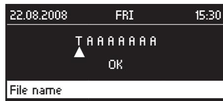
The file name consists of 8 letters or digits. Turn the control knob to select the desired letter or digit. Press the control knob to confirm the entry and move the cursor to the next position. After entry, press the knob again to confirm the name.
