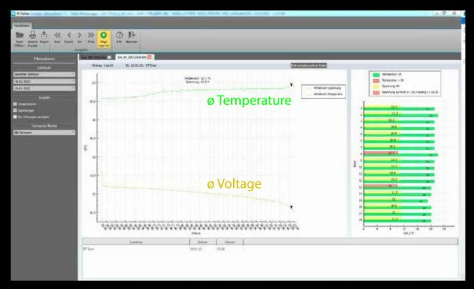
This log of a battery duration test clearly shows the sloping average voltage of the battery blocks (green) for the duration of the test. Exceedances of the limit values are indicated in red, this indicates the reviewing user directly the necessity of a battery check.
